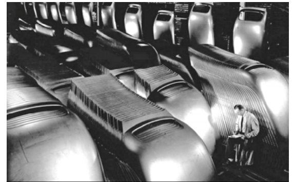
Stamped steel turret tops for different body styles in a Chevrolet body stamping plant.
