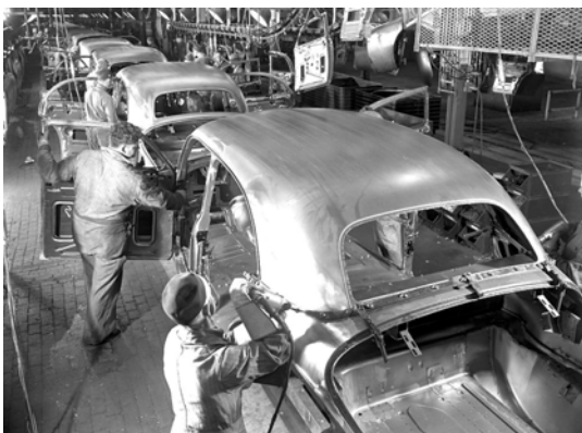
Stamped all steel turret tops on an assembly line in a Chevrolet body plant.
