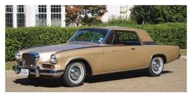
four bucket seats, and an aircraft-inspired cockpit. The base engine was a 240 bhp 289 ci V8, while a supercharged version provided 290 bhp. The car sold in limited numbers; 3,834 in 1963 and 4,445 in 1964, but it struck such a chord among enthusiasts that the Avanti outlived Studebaker itself!
